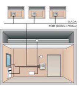
Regio Midi are controllers with a built-in sensor and an RS485 communication port. Controllers in different rooms can be connected to a bus line enabling communication with a central SCADA system via RS485 (EXOline or Modbus).
